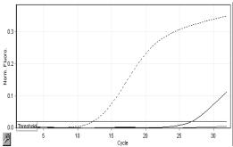
**Figure 1.** Result showing the amplification of one POSITIVE sample for MTB in Yellow (HEX) channel. Note: [Positive control (PC) is amplified (Ct 12.33) and Negative control (NC) is not amplified, which assertain the accuracy of the PCR run. The sample get amplified with Ct 26.82, at 0.02 threshold].
